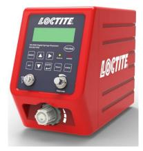
adhesive. The system can be operated in continuous, timer, cycle and program modes to dispense dots or beads. Suck-Back feature with digital vacuum display ensures no dripping.
